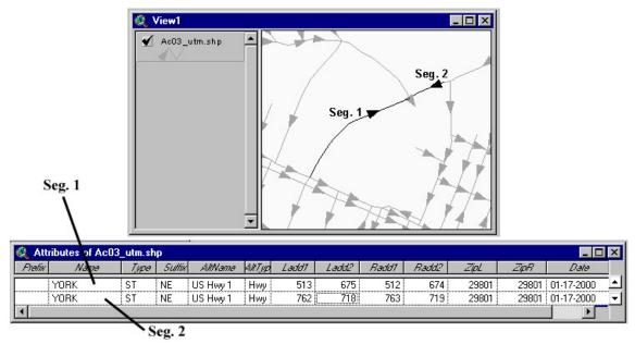
Example: Parity Correction by Changing Segment Direction
